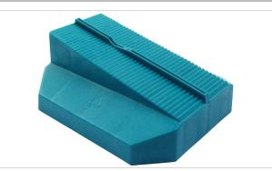
Combi Base is the basic component in the Combi series used for blocking up wooden floor on joists. The blocking up height ranges from 32-75 mm and further up to 250 mm when using Combi Extension. Combi Base is used together with Combi Top Small, Combi Top Medium or Combi Top Large. In addition, Combi Extension, Combi Sole, Combi Sound Reducer and Combi Sound Reducer Light can be used with Combi Base.
